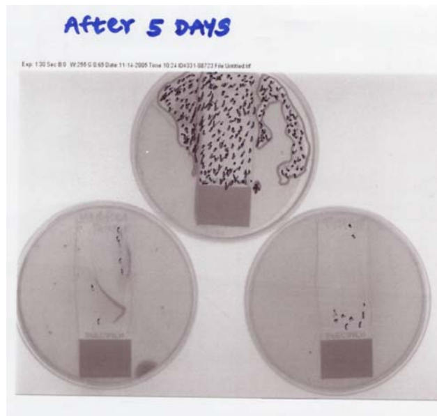
Figure 3.10 Bacterial growths on the blank, T 4 MPyP and modified T 4 MPyP coated slides after 5 days. The number of bacterial colonies on the T 4 MPyP and modified T 4 MPyP porphyrin coated slides was the same but the blank slide grew more bacterial colonies after 5 days.
