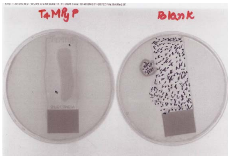
Figure 3.4 Growth of E-coli bacterial colonies on a blank slide and a slide coated with T 4 MPyP.
